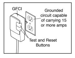
First, turn on the RENEW 207 by pressing the pump control on the console. Once the unit is running, press the GFCI "test" button. The spa should shut off. Press the "reset" button. The spa should resume normal operation. If the spa continues to run after the "test" button is pressed, the GFCI is damaged. Do not use the spa until the GFCI has been repaired or replaced by a qualified electrician.
